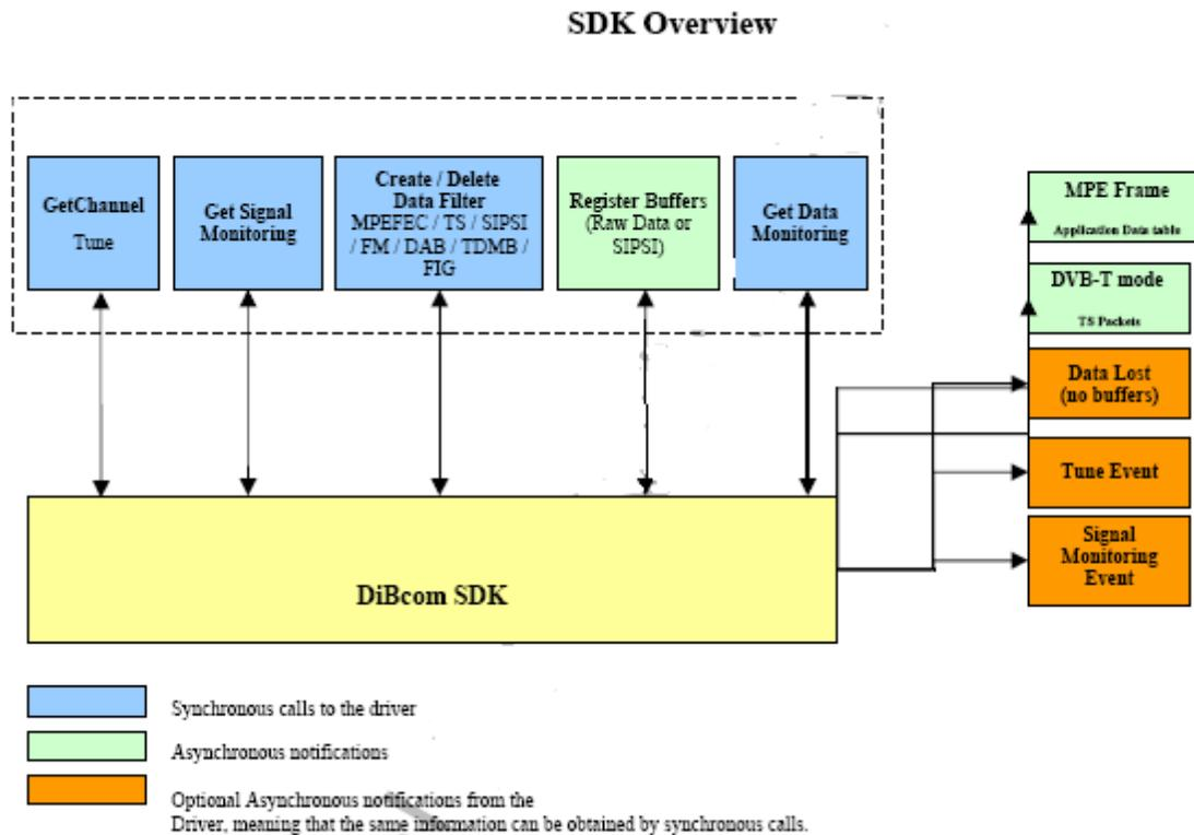
Figure 3: SDK for DIB9080H (provided by Dibcom)
