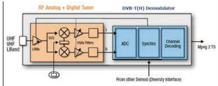
Figure 2: Block diagram of DIB9080H (provided by Dibcom)
