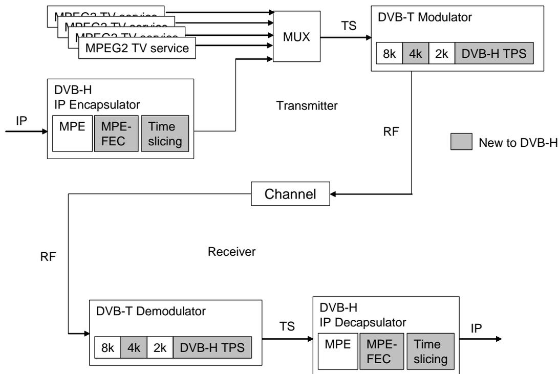
Figure 1. DVB-H link and physical layers
