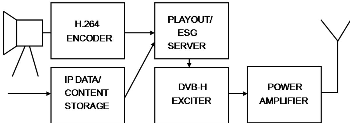
**Figure 6. TUT DVB transmitter system components**
