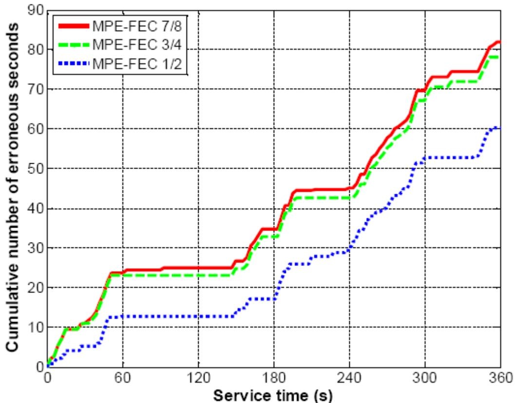
Figure 5. Cumulative number of erroneous seconds for a 256 kb/s streaming service across the measured trajectory with respect various MPE-FEC rates. [10]
