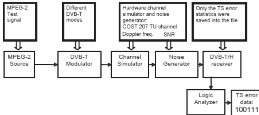
**Figure 3. Measurement setup for obtaining TS packet error traces [7]**
