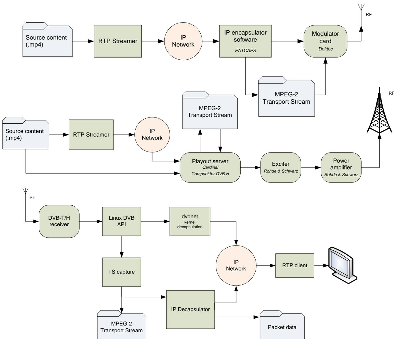
**Figure 3** DVB-H channel setup. Up: full-featured and PC-based transmitter; Below: Linux-based receiver.
