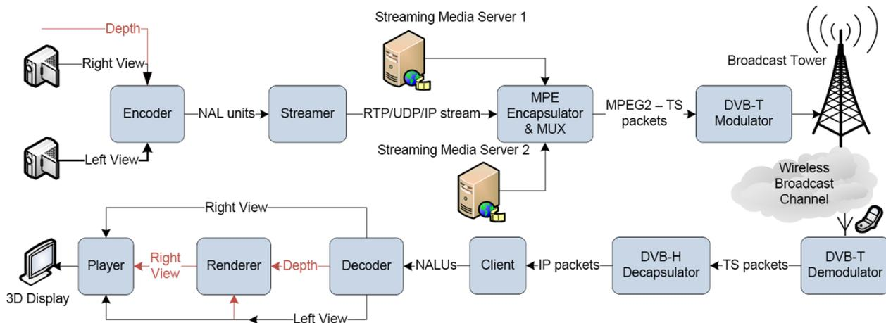
Fig. 3. Stereo-video broadcast over DVB-H channel
