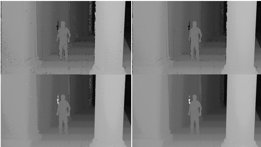
Figure 13. Depth estimation results for 'Dancer' dataset. From top clockwise: binocular; binocular with post-processing; trinocular with post-processing; trinocular.
