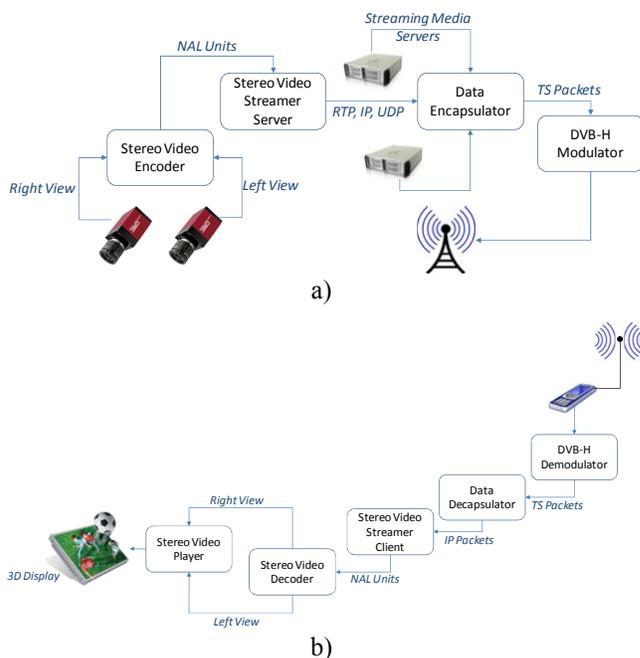
Fig. 1. Delivery of stereo video over DVB-H channel. a) Transmitter side; b) Receiver side.
