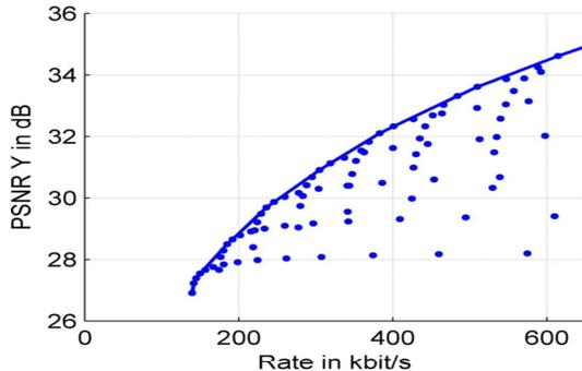
Fig. 7. Rate distortion points for different combinations of QPs for V+D. The envelop marks the optimal combination.
