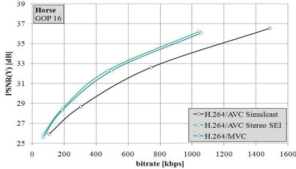
Fig. 6. Rate distortion curves for V+V encoding methods: H.264/AVC Simulcast, H.264/AVC Stereo SEI and H.264/MVC.
