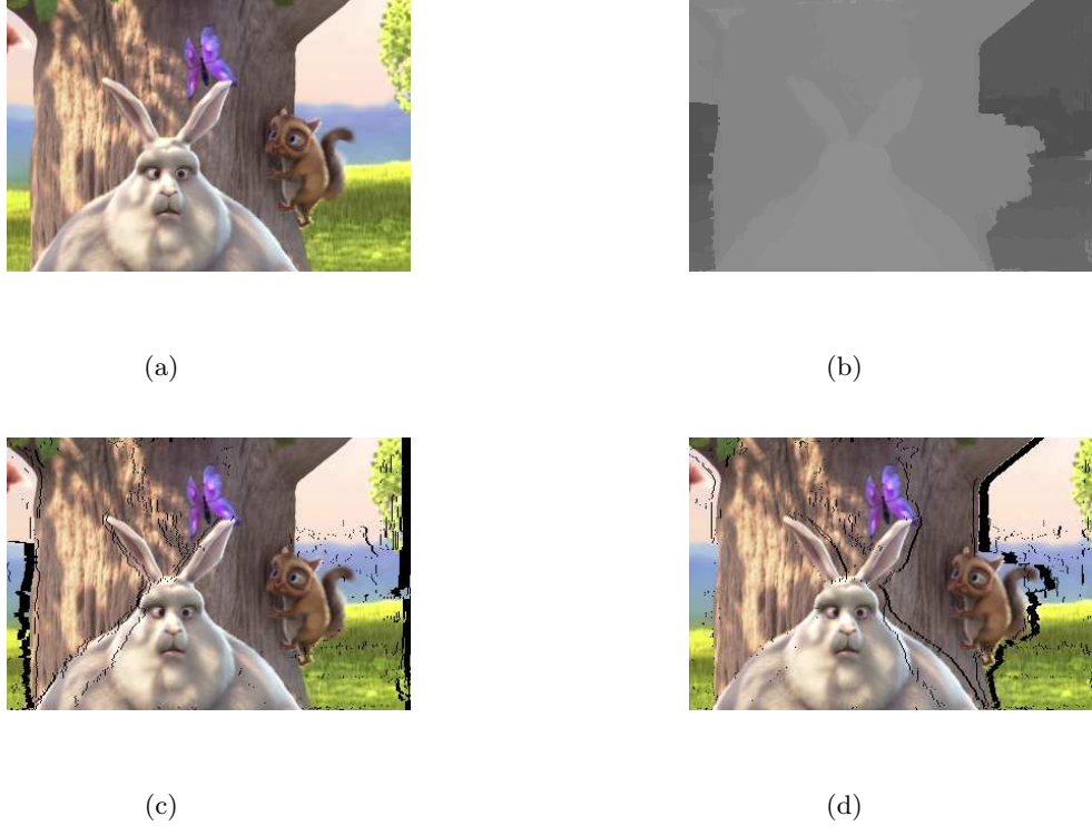
Figure 2. Example of an original image (a) and its depth map (b), and the corresponding left (c) and right (d) rendered images.
