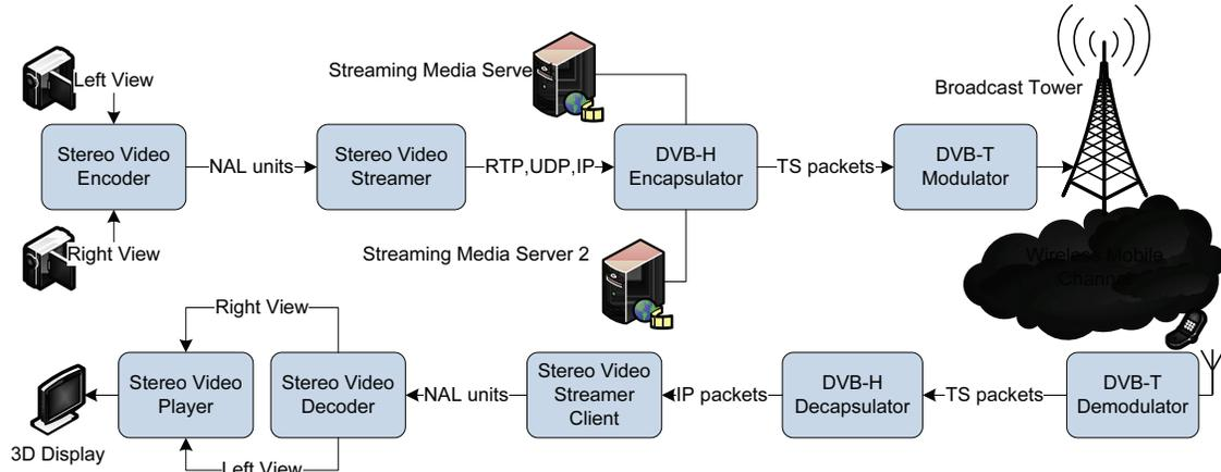
Fig. 1. Block Diagram of the End-to-End Stereo Video Transmission over DVB-H Simulation System.
