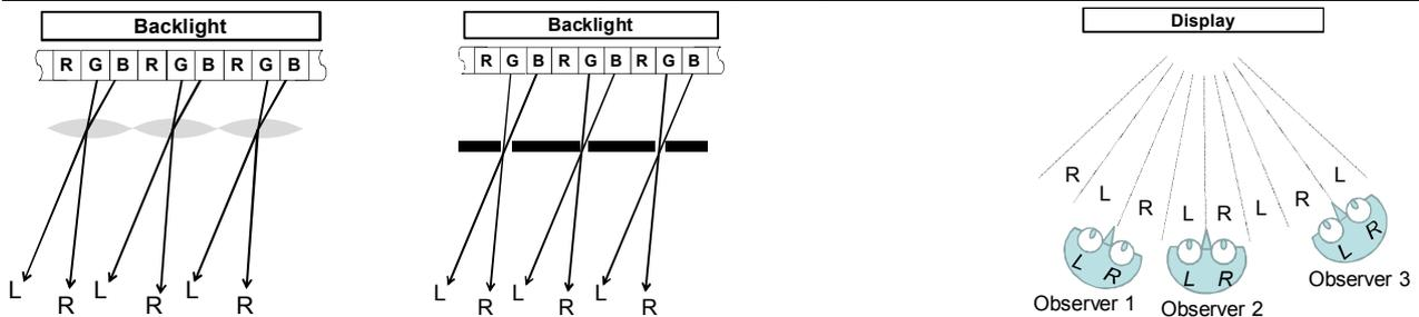
**Figure 1. Redirecting the light of an autostereoscopic display: a) lenticular sheet, b) parallax barrier, c) Observation**
