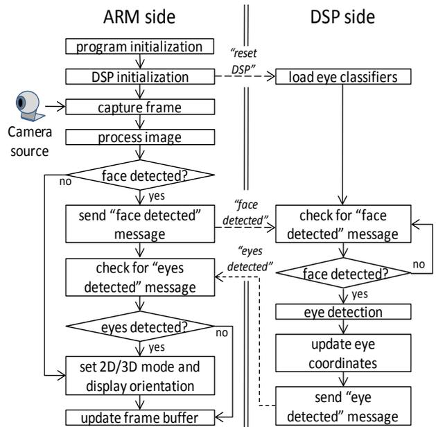
Figure 11. Application flow diagram of DSP and ARM.
