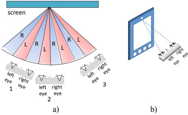
**Figure 2. Position of the observer in respect to the display: a) visibility zones of views and b) position of the user as detected by the front facing camera**
