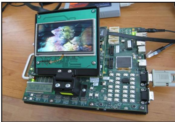
Fig. 5. Auto-stereoscopic display interface card for the OMAP 3430 SDP
